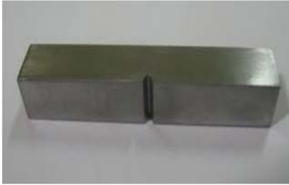
Figure 1: Grade 23a Stainless Steel Specimen used for Charpy Impact Testing (Francis, 2014).
